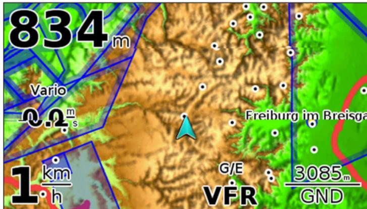
The **Airspace info** shows the **upper and lower limit as well as airspace classification** along with the corresponding rules (VFR / IFR) of the current airspace. This is generally G/E VFR (visual VFR flight permitted in accordance with the visual flight minimum of airspace G/E), as well as GND as the lower limit and current altitude of FL 100 (or FL 125/130/145) in meters above sea level.
